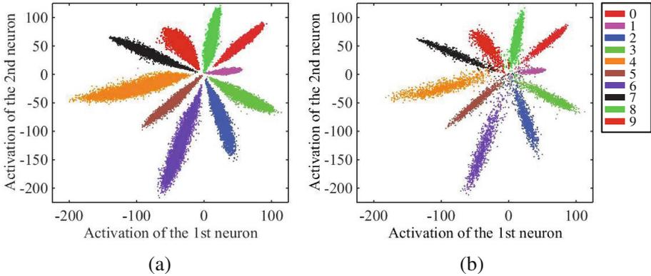
**Fig. 2.** The distribution of deeply learned features in (a) training set (b) testing set, both under the supervision of softmax loss, where we use 50K/10K train/test splits. The points with different colors denote features from different classes. **Best viewed in color.** (Color figure online)
