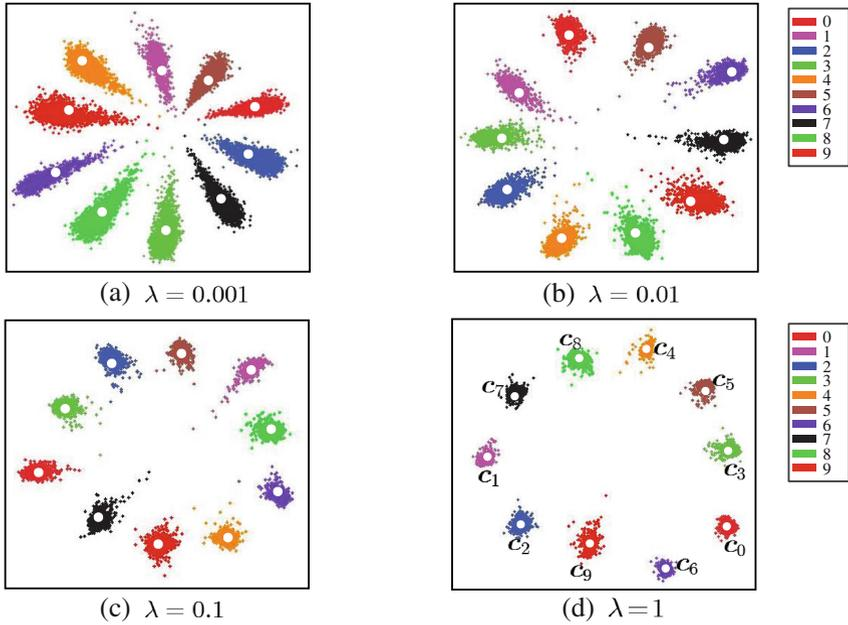
**Fig. 3.** The distribution of deeply learned features under the joint supervision of softmax loss and center loss. The points with different colors denote features from different classes. Different  $\lambda$  lead to different deep feature distributions ( $\alpha = 0.5$ ). The white dots ( $c_0, c_1, \dots, c_9$ ) denote 10 class centers of deep features. **Best viewed in color.** (Color figure online)
